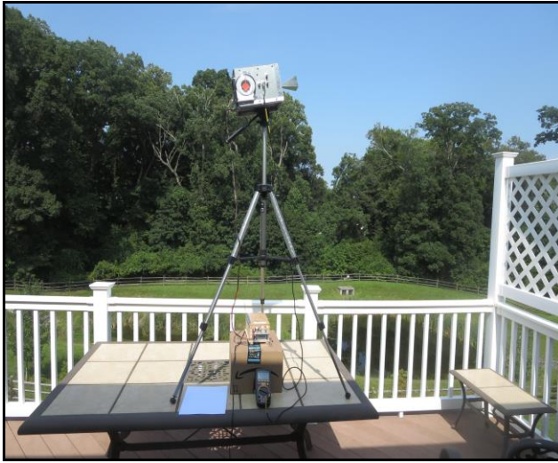
Figure 39- Clear sky tipping curve measurements of the 20 GHz radiometer made August 26, 2018. Unfortunately, blockage of the sky radiation at low elevation (large zenith angle) occurs by the surrounding trees, house and privacy panel. To minimize blockage the radiometer is mounted on a tripod that is elevated on a table. The right picture shows the view seen by the radiometer when the antenna views at low elevation. Observations for zenith angles greater than 70^\circ are obstructed by the trees and house shown in the picture.
