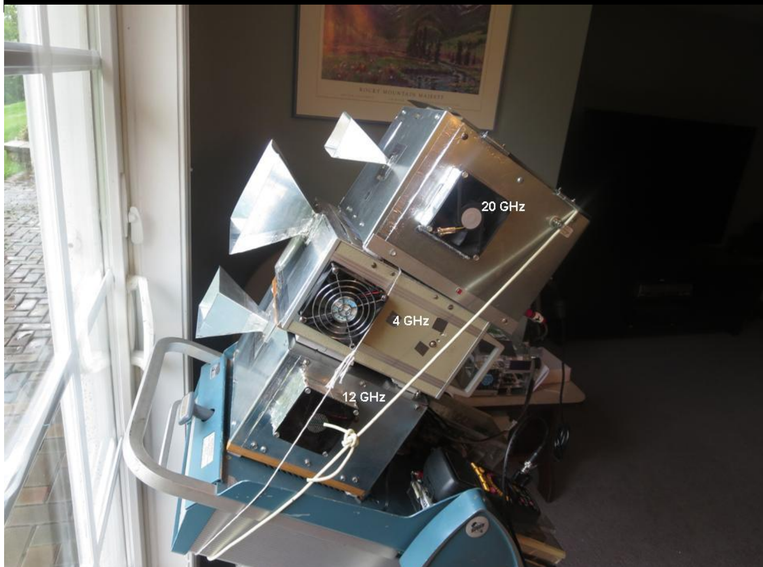
4 GHz, 12 GHz and 20 GHz radiometers viewing rain through a glass patio door
