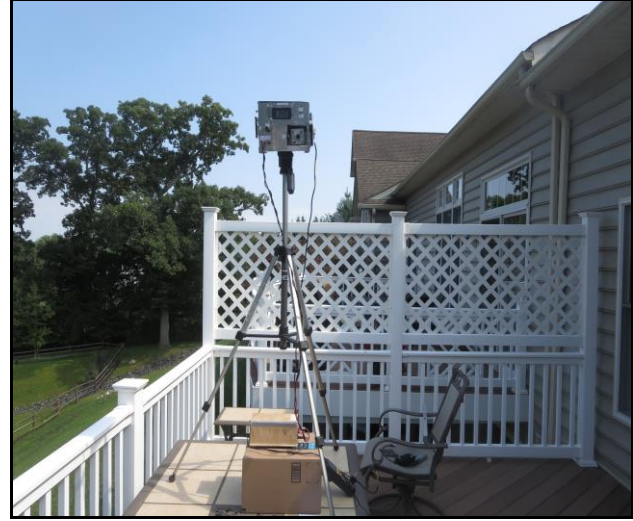
Figure 39- Clear sky tipping curve measurements of the 20 GHz radiometer made August 26, 2018. Unfortunately, blockage of the sky radiation at low elevation (large zenith angle) occurs by the surrounding trees, house and privacy panel. To minimize blockage the radiometer is mounted on a tripod that is elevated on a table. The right picture shows the view seen by the radiometer when the antenna views at low elevation. Observations for zenith angles greater than 70^\circ are obstructed by the trees and house shown in the picture.
