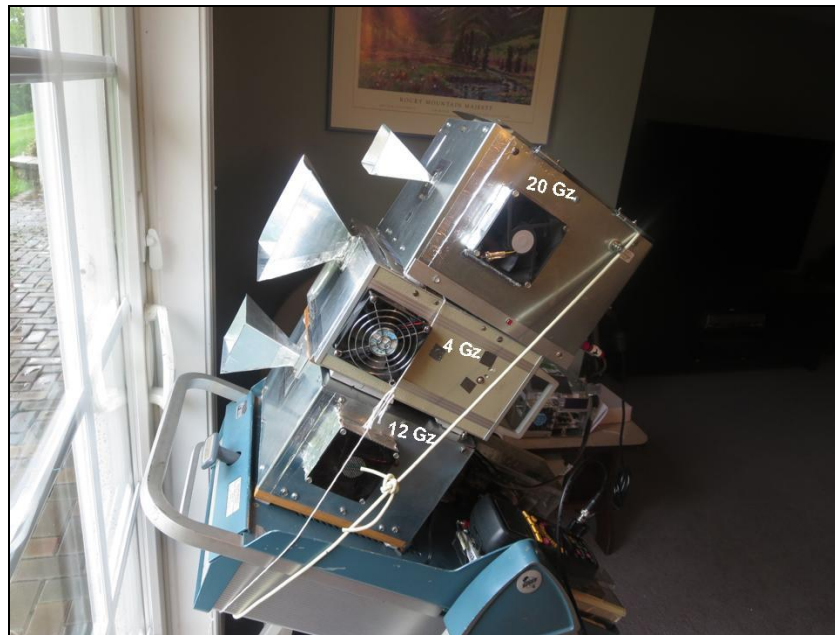
Figure 28- The 20 GHz radiometer is mounted on top of the 4 and 12 GHz radiometers. The 20 GHz radiometer has the smallest antenna with 20 dB gain. In comparison, the 12 GHz antenna has 19 dB gain while the largest antenna at 4 GHz has the smallest gain of 15 dB.
