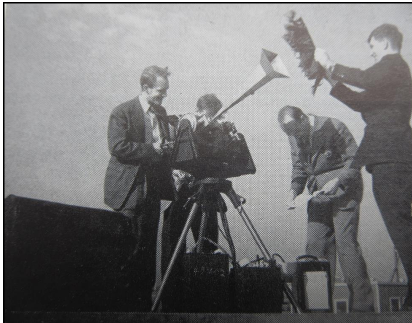
Tipping curve absorption measurements made in 1946 by Dr. Robert Dicke along with his associates. Starting on the Left is E. Beringer, R. Kyhl, A. Vane and R. Dicke. This picture is in the MIT Rad Lab Book "Five Years" (see pg. 113). It shows Dicke holding up an absorber in front of one of his radiometers while a chart recorder on the ground plots the measurements.
